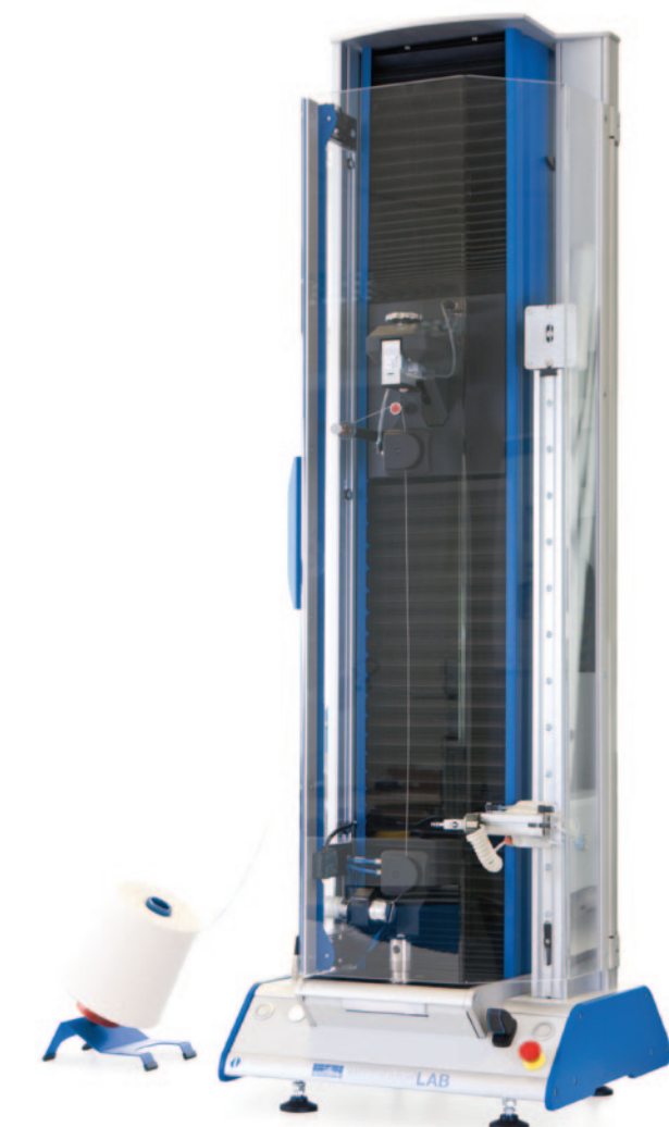
Example of yarn traction
