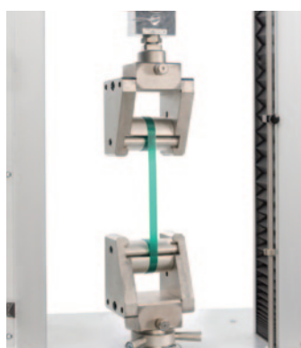
Self-tightening high tenacity clamps for ribbons, 100 mm wide, Code 2512E.920
