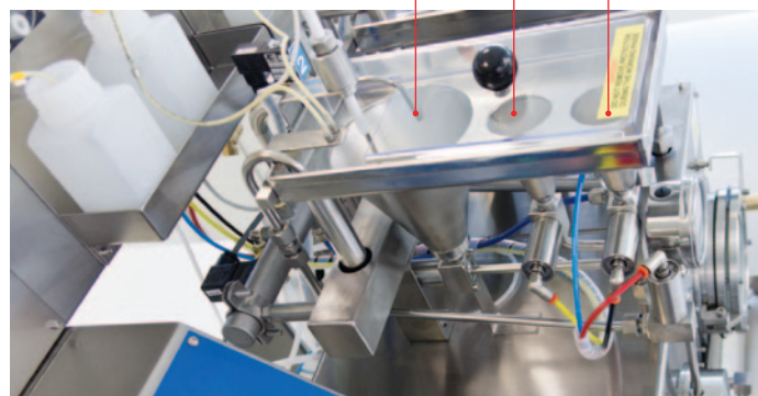
Picture showing the 3 automatic dosing tanks.
