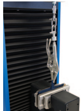
Upper Long Nose Vise Grip, for trousers' hooks and other accessories, according to M&S P115 (for buttons), Code 2510.152
