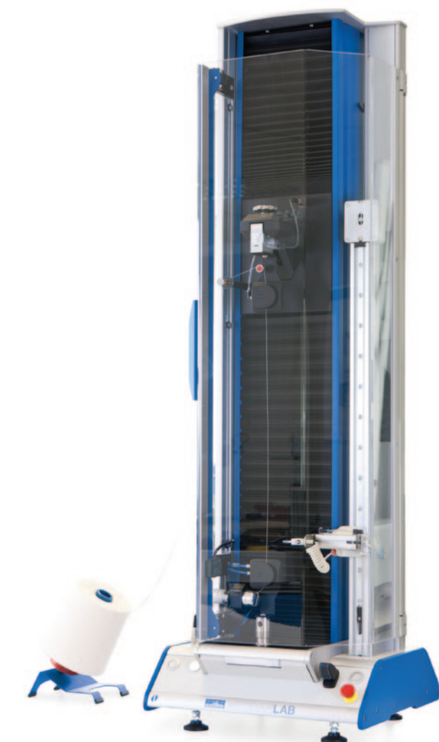
Example of yarn traction
