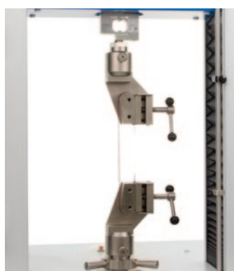
Mechanical clamps for high tenacity yarns, Scott 300, Code 2510.996
