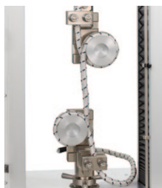
Self-tightening high tenacity clamps for ropes, Code 2515.988
