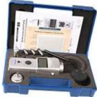
Tachometer with 2 batteries, carrying case, 1 adapter H, 2 rubber tips, 1 funnel, 1 measuring wheel with 6 inch circumference, 1 extension, 1 page reflective tapes (35 pieces), Certificate of Compliance with the order 2.1 according EN 10204 free of charge and operating instructions in german and english
