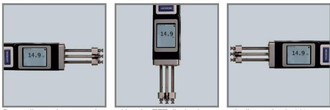
Depending to the measuring position the TFT display is automatically rotating in 90° steps
