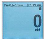
Automatic "Zero-Setting" in each measuring position using a special sensor technique. 4 Material memory locations for customer made calibrations.
