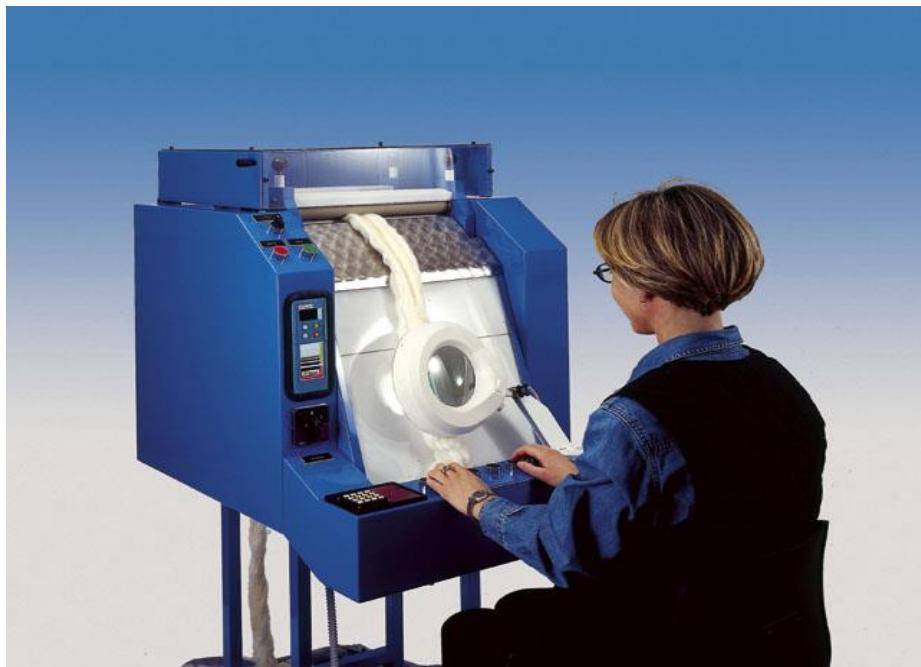
An instrument to count impurities and neps in wool, cotton and synthetics tops. It is designed for quick and accurate counting of impurities. Adjustable speed from 5 to 12 m/min, adjustable distance between rollers from 42 to 260 mm, predetermined drawing standard value: 6.35. Includes a series of six electronic counters for counting and classification of different impurities.
