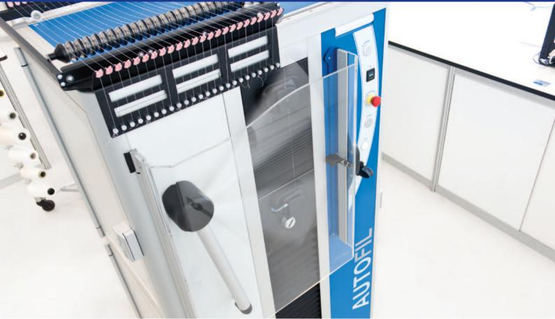
Fully automatic 24-position **yarn** strength tester. It can test **hanks** and **fabrics** as well in the semi-automatic mode.
