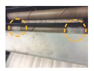
CONTEST-S makes the difference in the working principle, since it provides a counting per gram of the sticky points and their sizes by simulating the carding process like in a real spinning process.
