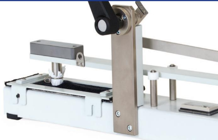
Suitable to measure color transfer/staining on any kind of knitted or woven fabrics, labels, narrow fabrics, carpets, sewing threads, etc.
