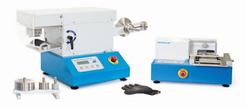
Compact and user-friendly benchtop instruments to determine the resistance to cutting by sharp objects, in compliance with the main international Standards. Particularly recommended to measure the resistance to cutting of PPE (Personal Protective Equipment) like protective gloves and clothes.
