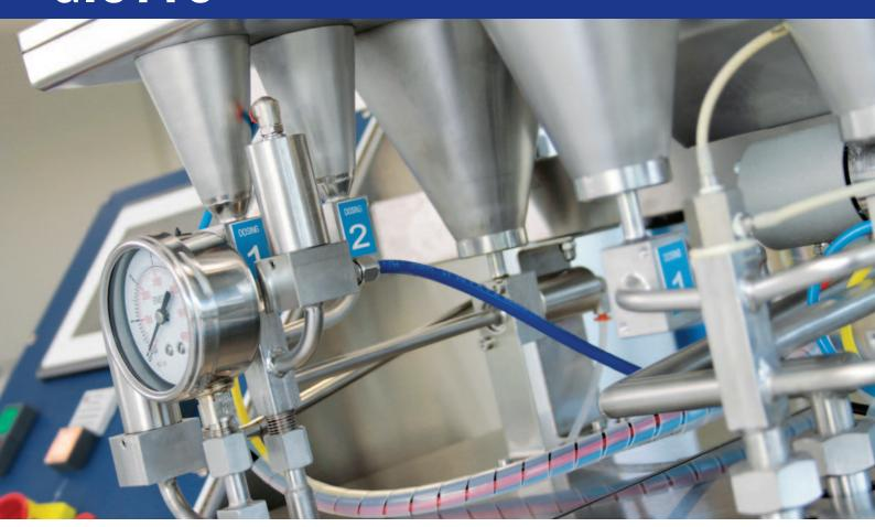
Miniature Laboratory PILOT piece dyeing machine, replicates Bulk Dyeing and fills the void between regular IR Lab dyeing machine and bulk production machine.
