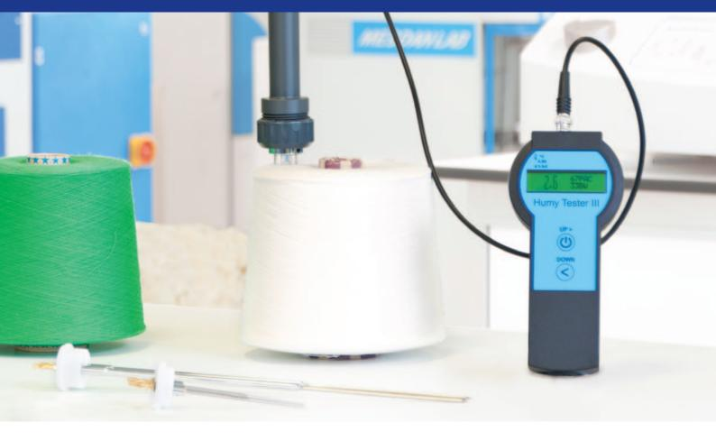
Multifunctional portable digital instrument for the instantaneous reading of moisture in textile materials (bales, slivers, yarns, fabrics) as well as of ambient temperature and RH%.
