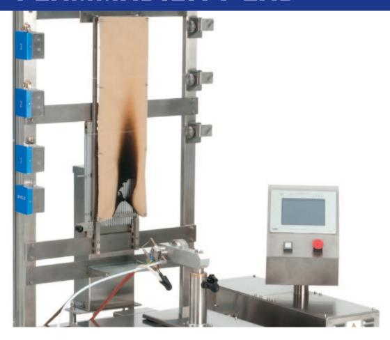
Multipurpose instrument to measure the textile resistance to flame propagation and to observe specimen behaviour to flame like the assessment of debris and its conditions (ash, glowing particles).
