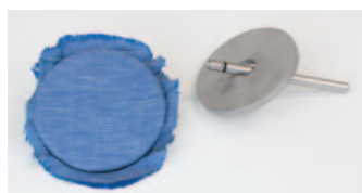
Example of 1-position sample holder with Ø 90 mm
