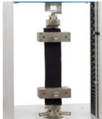
Mechanical clamps with rubber jaws, 100 mm wide, Code 2510.846
