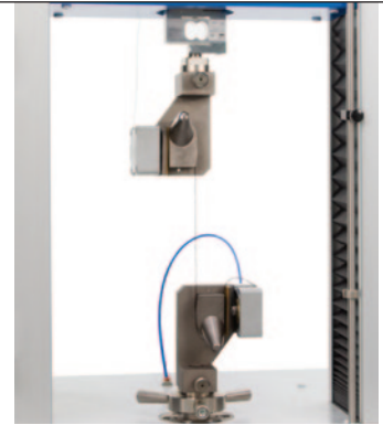
Clamps for high tenacity yarns with conical introducer, Code 2510.980
