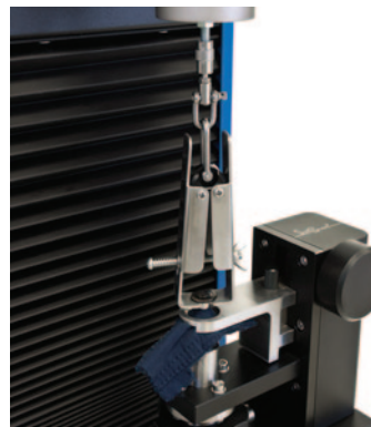
Upper ( Code 2510.155 ) & Lower ( Code 2510.154 ), Grasp Button Kit, & Lower Fabric Clamp ( Code 2510.150 ), for buttons, etc.
