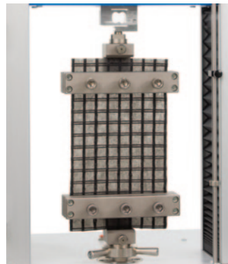
Mechanical clamps for non-woven and geo-textiles, (EN ISO 10319), 200 mm width, with rubber jaws, Code 2515.142
