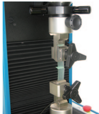
Mechanical PBF Clamps for films, width 25mm, Code 2512A.997
