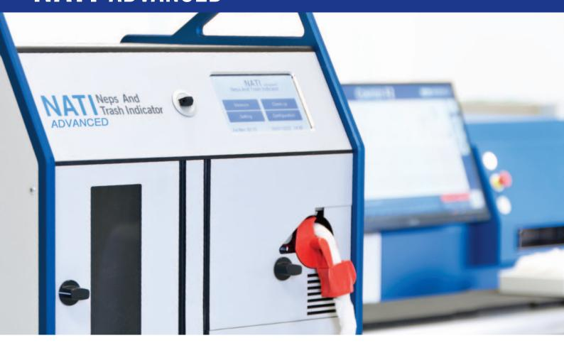
NATI was designed to measure and classify neps & trash, to improve & predict yarn quality, to increase efficiency of carding & combing operations, to reduce maintenance costs and overheads. Its usefulness in programming card-clothing grinding and card-wire replacement is beyond compare.
