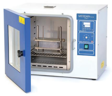
Instrument to check the colour fastness of textiles and leather to water and perspiration under the action of different agents such as:
