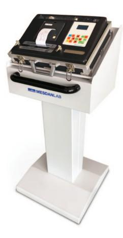
· Data output: force, elongation, tenacity (RKM) and the relative statistical analysis (min, average, max. CV%, etc.). Data are displayed on the screen, printed by the built-in printer, and saved on a USB flash memory.
