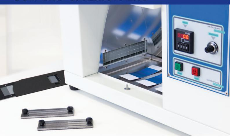
Compact and user-friendly bench-top instrument designed to test color fastness to light exposure.
