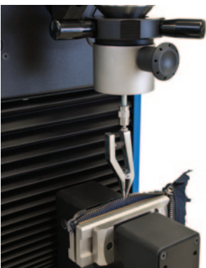
Element for Zipper Kit ( Code 2510.157 ), in compliance with ASTM D2061 Standard
