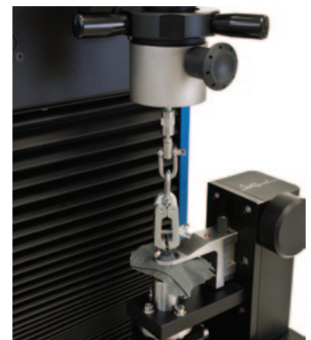
Upper Stud Grip ( Code 2510.153 ), Lower Fabric Clamp ( Code 2510.150 ), to test male parts of baby snaps, etc.
