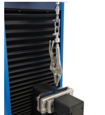
Upper Long Nose Vise Grip, for trousers' hooks and other accessories, according to M&S P115 (for buttons), Code 2510.152
