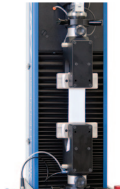
Pneumatic Clamps for medium-heavy fabrics, up to 300 Kg capacity approx., 100 mm width, Code 2512E.730 *
