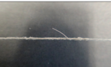
Lycra core protrusion
