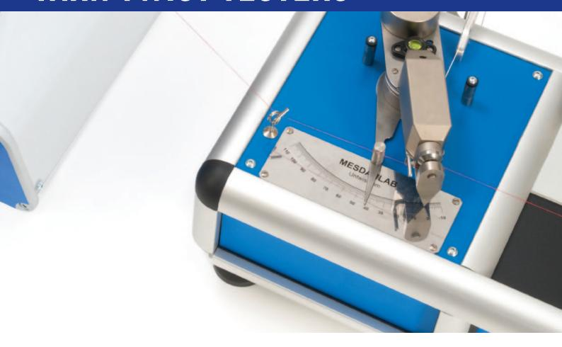
The measurement of the number of yarn twists and their uniform distribution within a package is an essential parameter of yarn quality and final fabric quality. In order to meet different requirements in terms of automation and costs, Mesdan Lab is offering a wide range of yarn twist testers:
