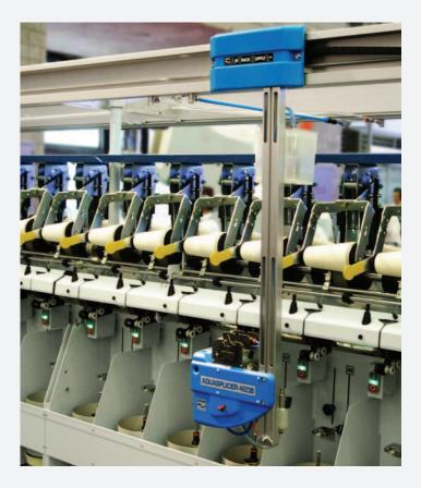
ATS "L" type fitting AQUASPLICER 4923B installed **on two-for-one twisting machine** processing fine plied compact cotton yarns.
