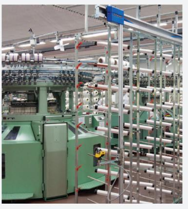
ATS "C" type with JOINTAIR 110R installed on the creel of a circular knitting machine.
