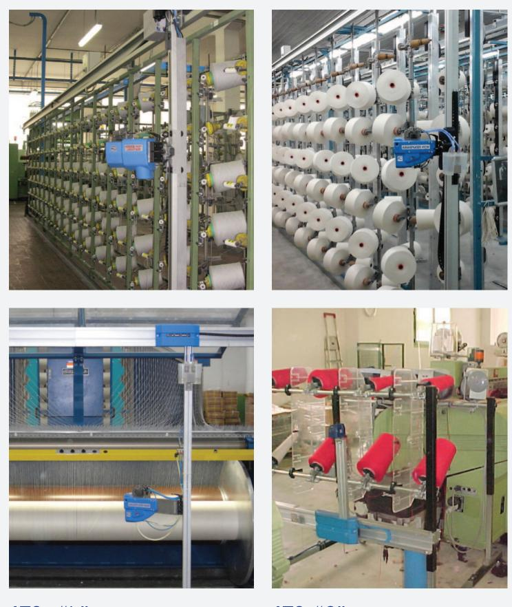
ATS "L" type with AQUASPLICER 4923B placed in front of a fractional warping machine for cotton yarns. ATS "C" type with JOINTAIR 115 fitted on weft weaving creel for top-to-tail join.
