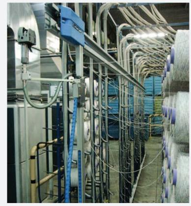
ATS "C" with floor guide fitting JOINTAIR 116 on a sliding bar with swivel joint enabling splicer vertical movement on the **Tufting creel**.
