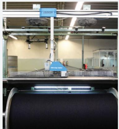
ATS "L" with INDIGO SPLICER 4662 installed on a **Rebeamer** - downstream of rope dyeing.
