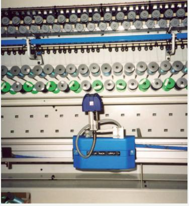
JOINTAIR 115 ATS "C" type with JOINTAIR 115 on embroidering machine.
