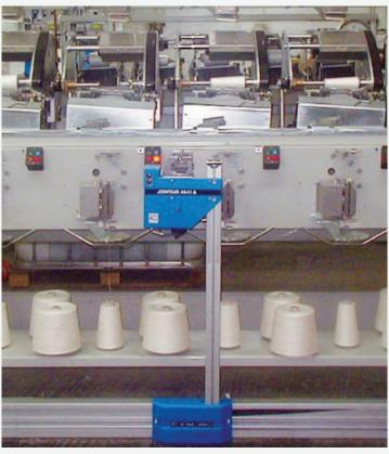
JOINTAIR 4941A ATS "L" type with JOINTAIR 4941A on finishing winder processing sewing threads.
